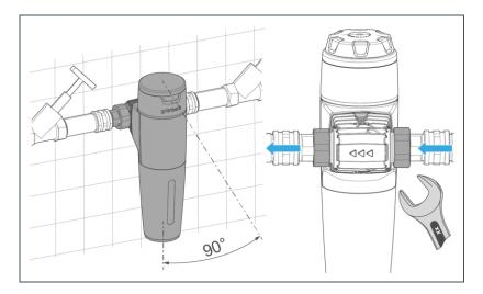
**5.** Tighten the click-type connection flange with the union nuts without applying tension.
