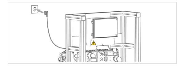
▶ Plug the power plug into the 230 V socket.
