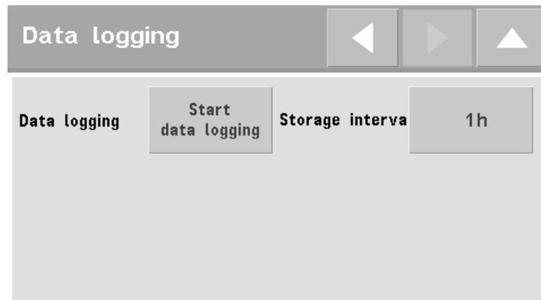
Recording begins once the "Start data logging" button has been pressed; the button text then changes to "Stop data logging." The logging interval can be set using the "--h" button.
