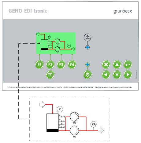
Fig. F-20: Visualisation system of the PB system
