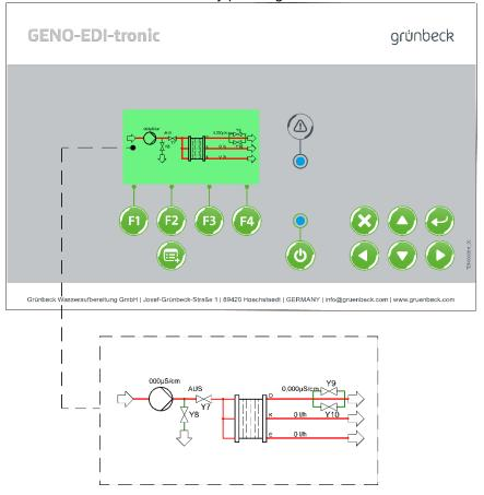
Fig. F-12: Visualisation system of the GENO-EDI-X system
