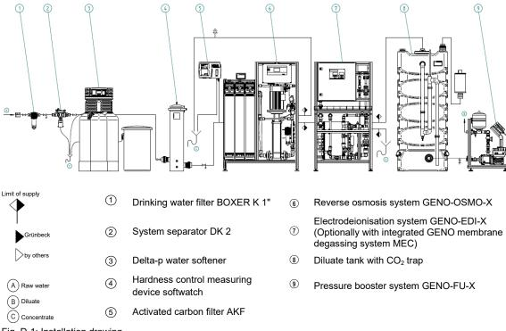
Fig. D-1: Installation drawing
